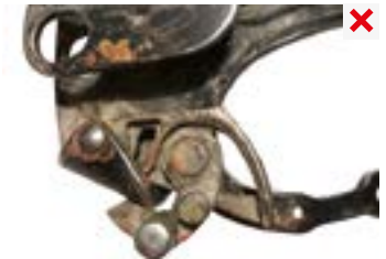
corroded - functionality limitation
