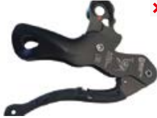
damaged regulation handle
